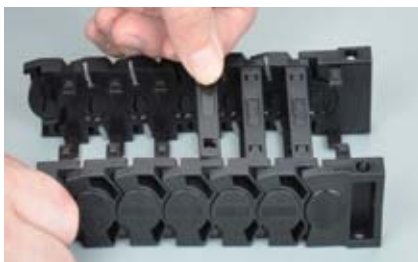
Assemble crossbars - push down and snap from one side
