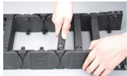
Assemble crossbars - push down and snap from one side
