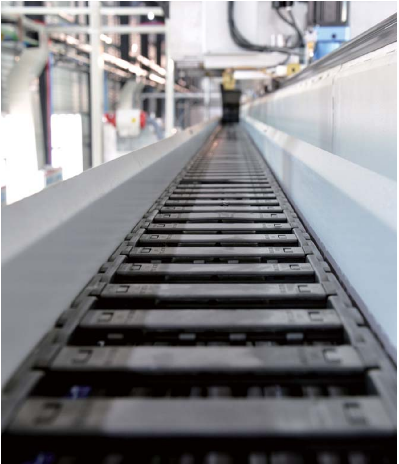
C03 cable carriers protects long-stroke robot cables
