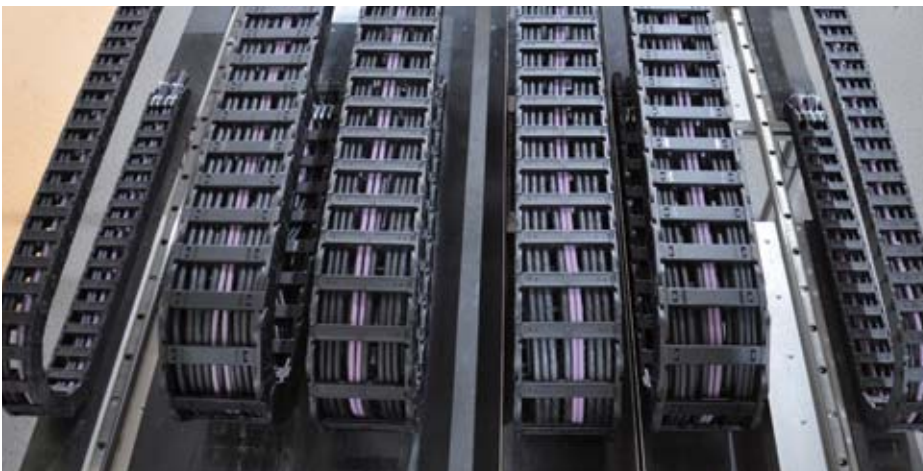
Short-travel unsupported durability test for flexible cables and cable carriers
