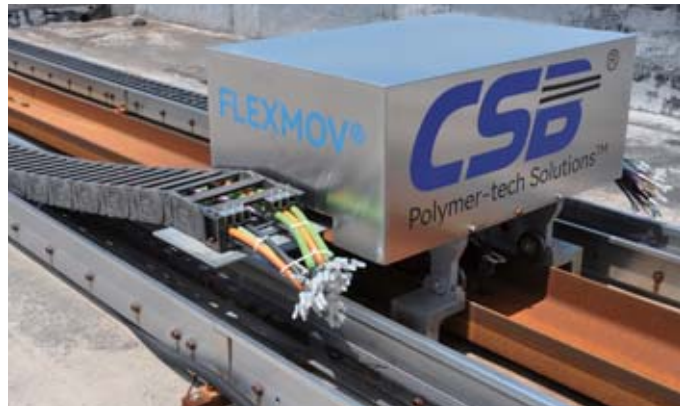
Long-travel outdoor sliding durability test for flexible cables and cable carriers
